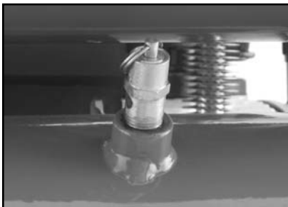
Figure 8. Safety drain valve.
